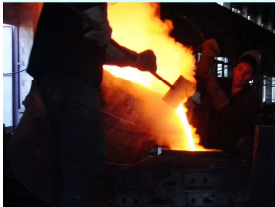
Copper shielding was cast in Armenia.
