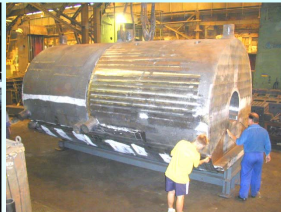
100 tonne heavy iron pieces were cast in the Czech republic.
