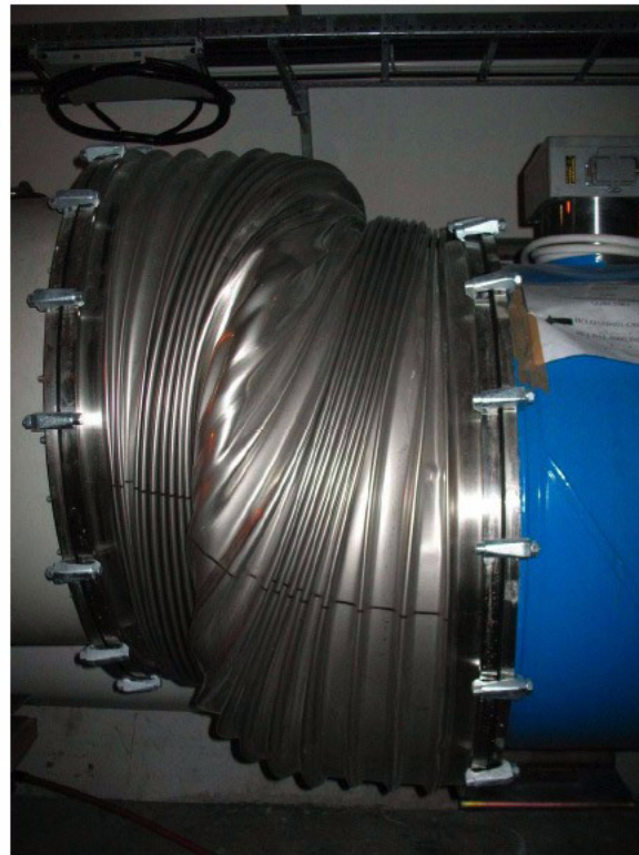
Figure 41: Damage of the LHC magnets in sector 3-4 of the LHC, caused by the incident of 19 September 2008
