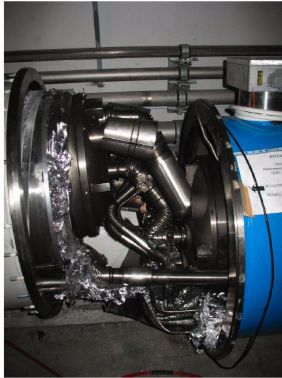
Figure 41: Damage of the LHC magnets in sector 3-4 of the LHC, caused by the incident of 19 September 2008
