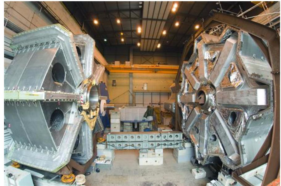
Figure 71: ATLAS solenoid (left) and end-cap toroid (right)
