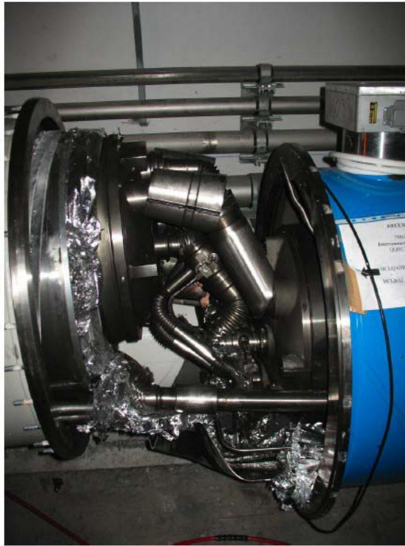
Figure 35: Damage of the LHC magnets in sector 3-4 of the LHC, caused by the incident of 19 September 2008
