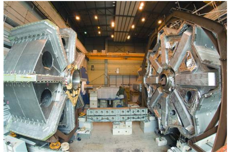
Figure 65: ATLAS solenoid (left) and end-cap toroid (right)
