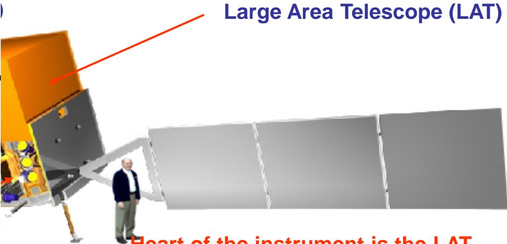
Heart of the instrument is the LAT, detecting gamma conversions
