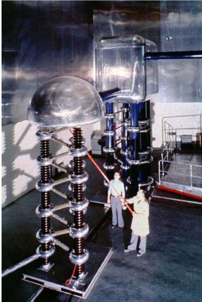
Figure 19: The Cockcroft-Walton “generator” at CERN: accelerates particles by an electrostatic field
