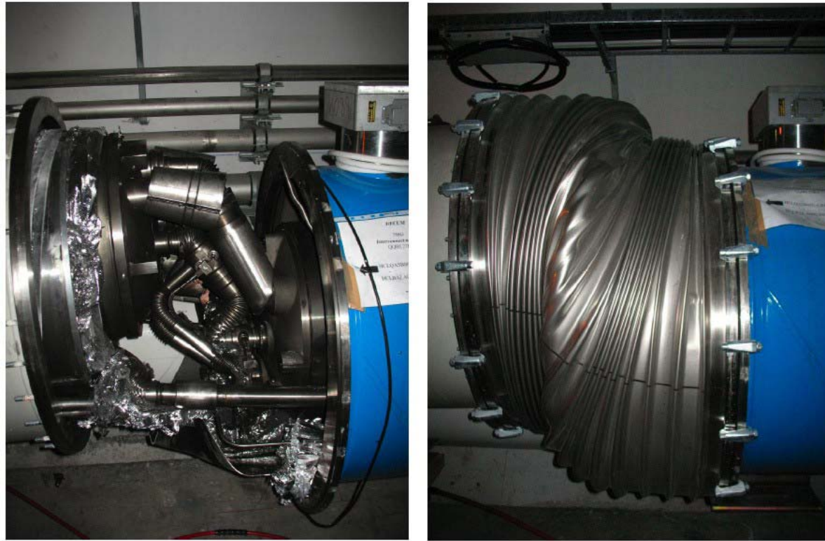
Figure 35: Damage of the LHC magnets in sector 3-4 of the LHC, caused by the incident of 19 September 2008
