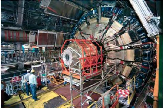
Figure 5. The insertion of the SCT and the TRT Barrel in the Barrel Calorimeter.
