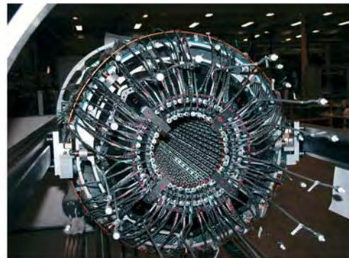
Figure 4. The Pixel Barrel layers 1 and 2.
