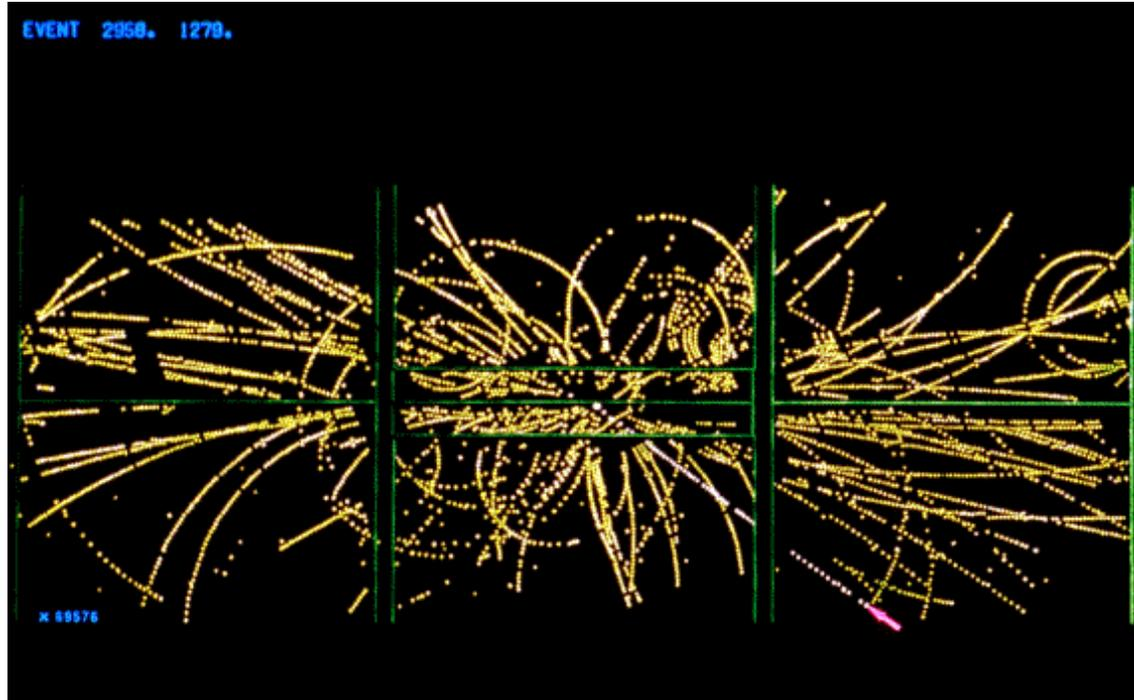
Figure 83: A W boson observed by UA1 detector in 1982; a high transverse momentum electron is indicated by the arrow
