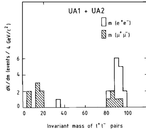
Figure 106: W and Z masses as measured by UA1 (W) and UA1 and UA2 (Z) experiments
