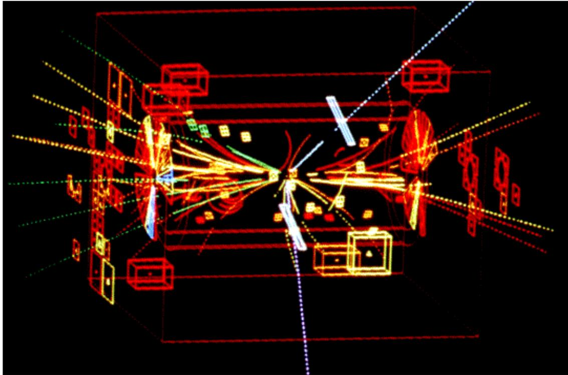
Figure 85: A  $Z^0$  production event in the UA1 detector.
