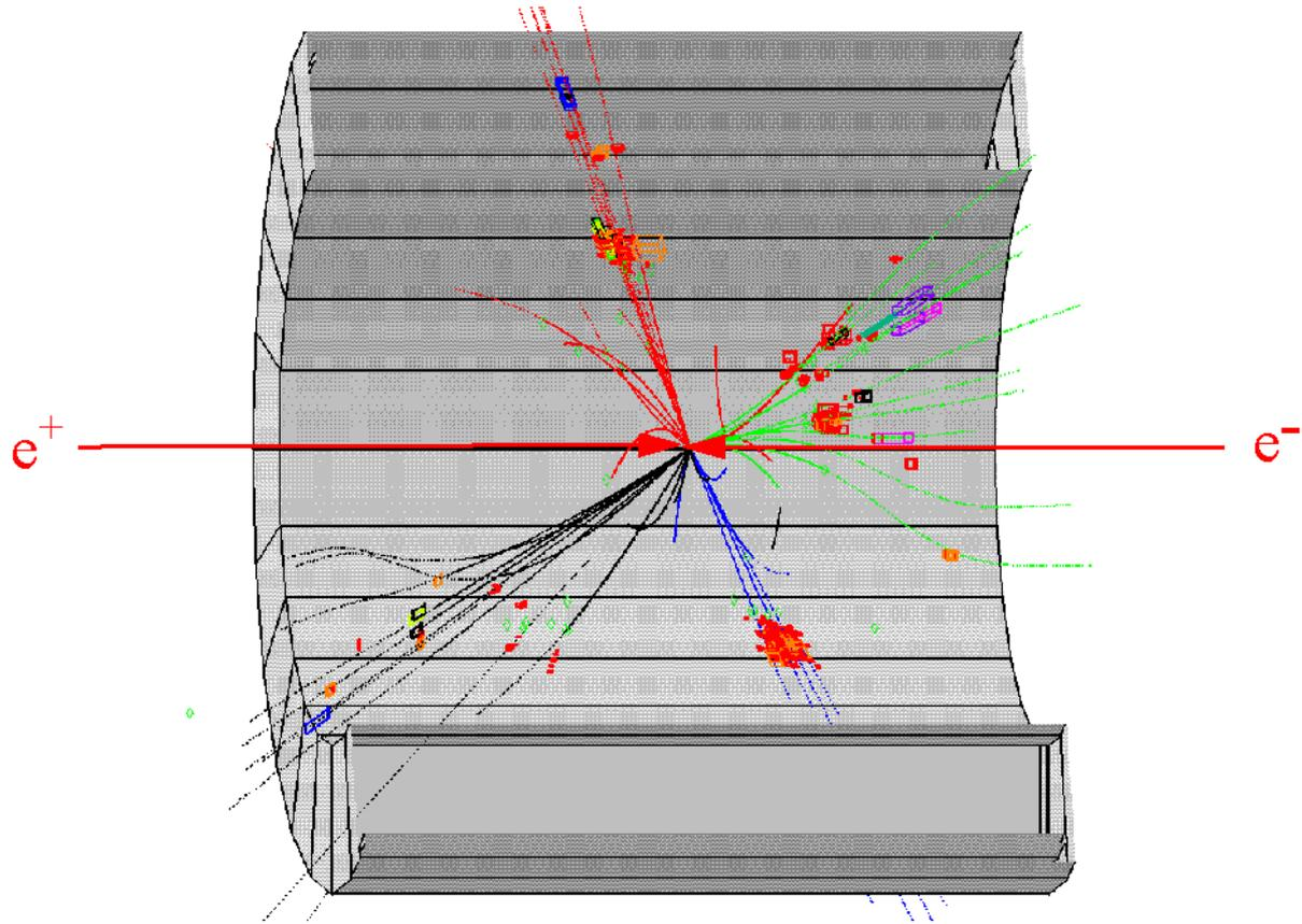
Figure 109: A 4-jet WW event as registered by the DELPHI detector at LEP
