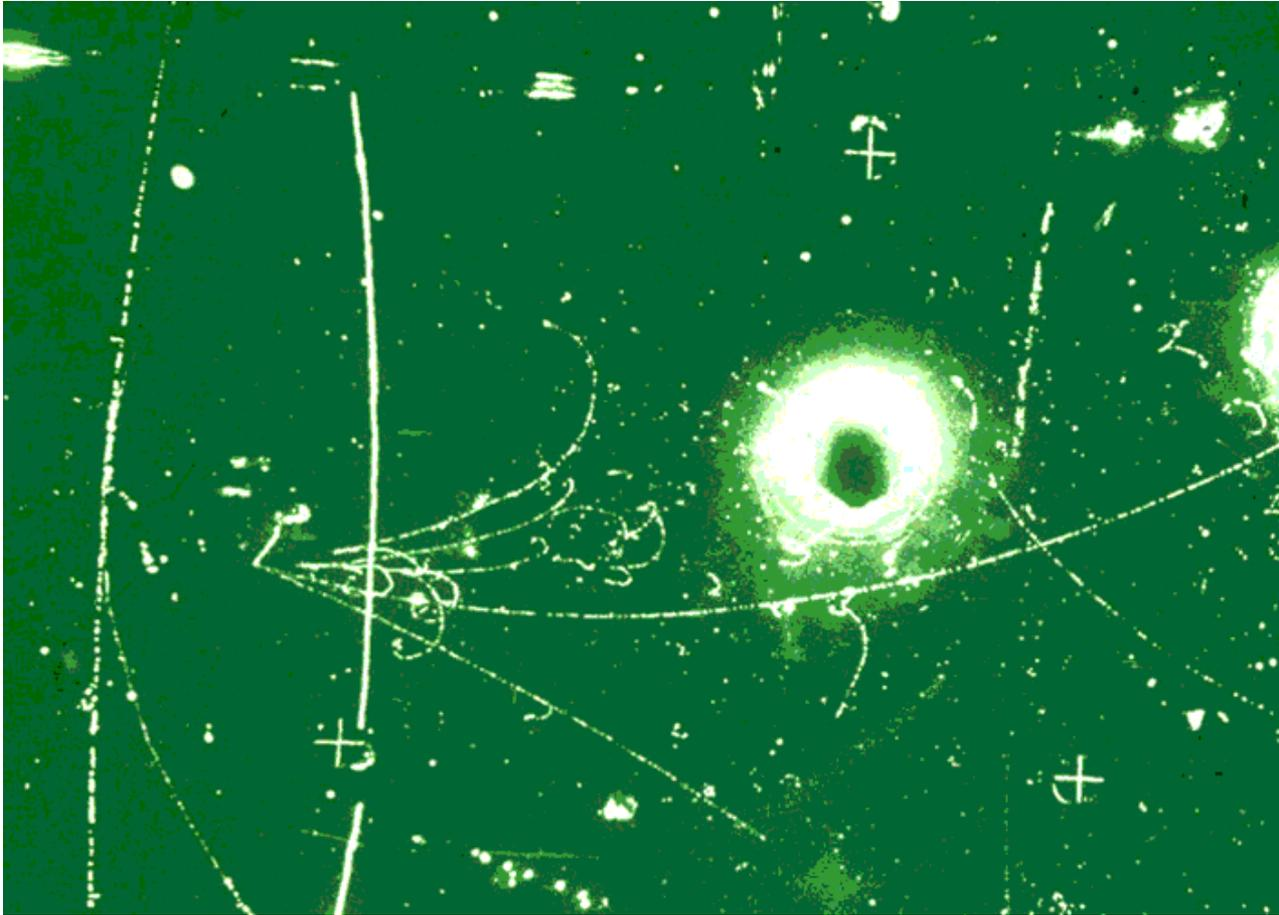
Figure 81: One of the first neutral current reactions as seen by the Gargamelle bubble chamber in 1973
