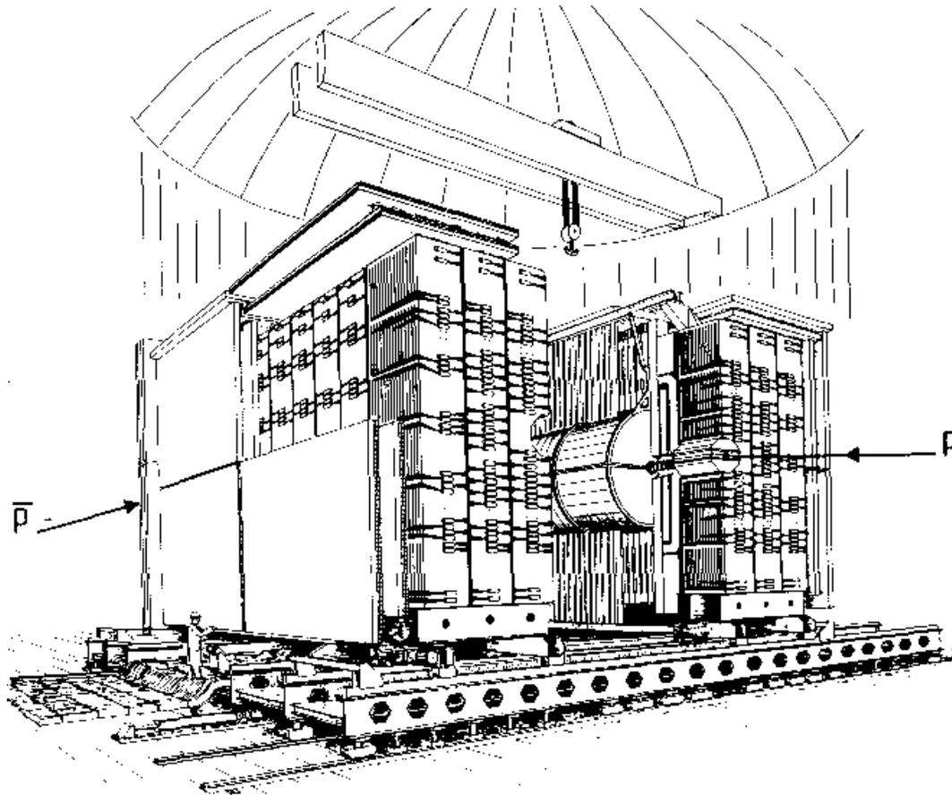
Figure 104: UA1 detector layout (proton-antiproton collisions); solid angle is fully covered down to  $0.2^\circ$
