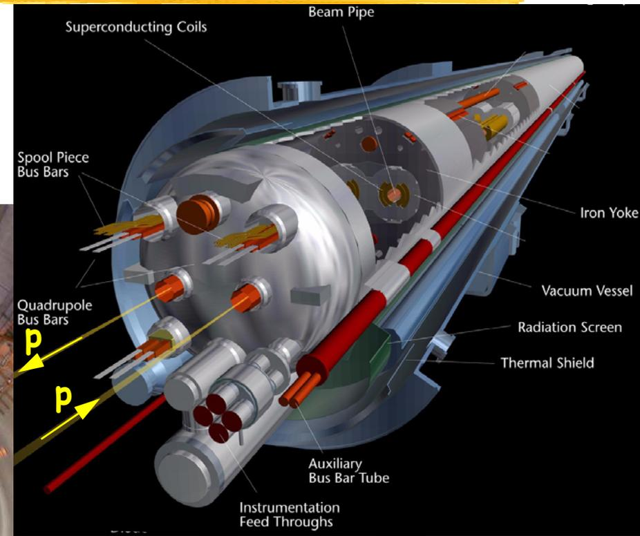
The current in the superconducting magnet coils is 11800 Ampere.
