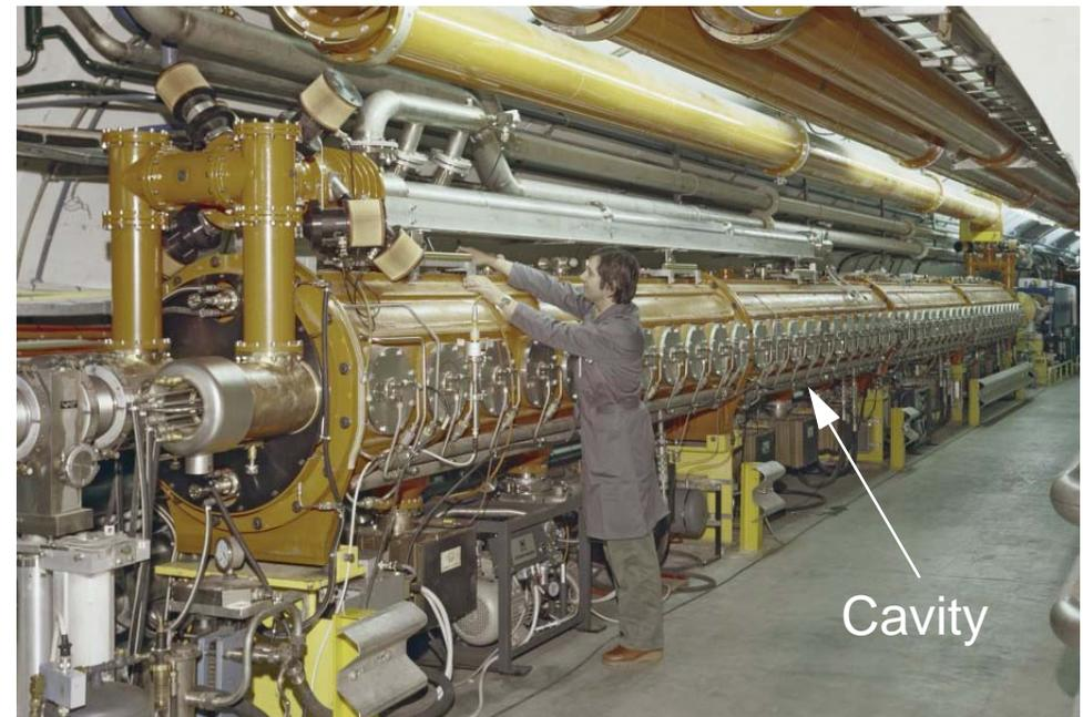
The SPS was originally a 450 GeV fixed target machine but was later converted to a collider with protons colliding with anti-protons. The accelerator is 6.9 km long and has 744 dipole magnets and 216 quadrupole magnets. The acceleration is given by 4 cavities operating at 200 MHz.
