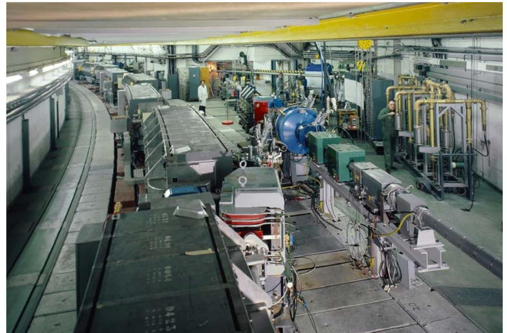
The PS accelerator is 628 m long and has 277 magnets (including 100 dipole bending magnets). It can accelerate protons to 28 GeV.
