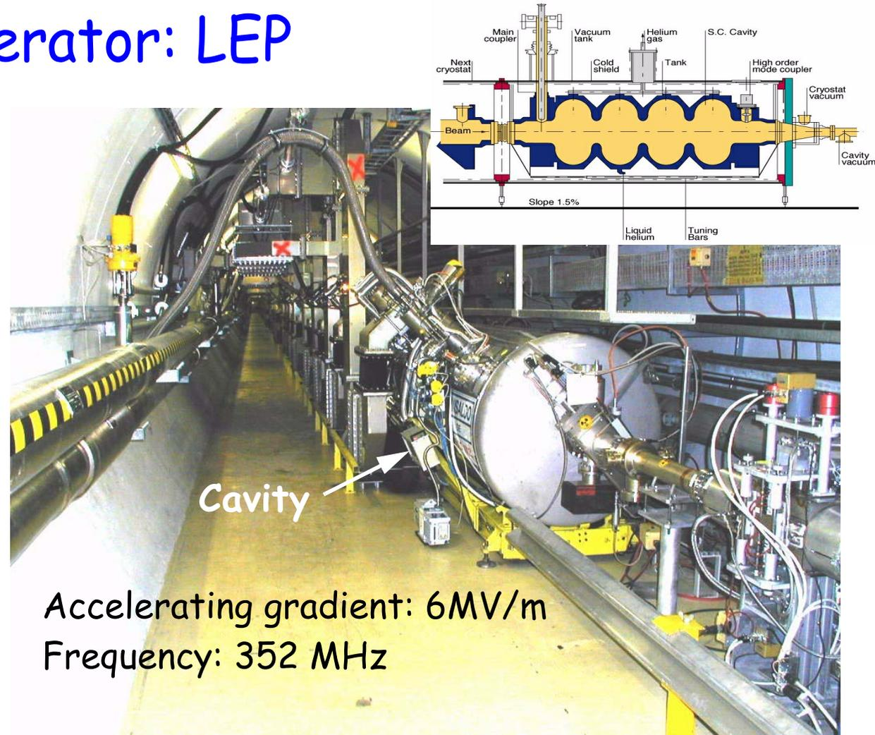
In a **first stage** the collision energy was equal to the Z mass (**91 GeV**) but it was increased in a **second stage** to **209 GeV** by installing 288 superconducting cavities.
