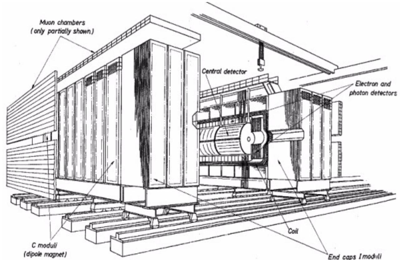
The UA1 detector had a **central wire chamber** that could measure tracks. A **dipole magnet** produced a 0.7 T field perpendicular to the beam direction. The **electromagnetic calorimeter** was of **lead/scintillator** type and the **hadronic** was an **iron/scintillator sandwich**. The **muon detector** consisted of 8 planes of **drift chambers**.
