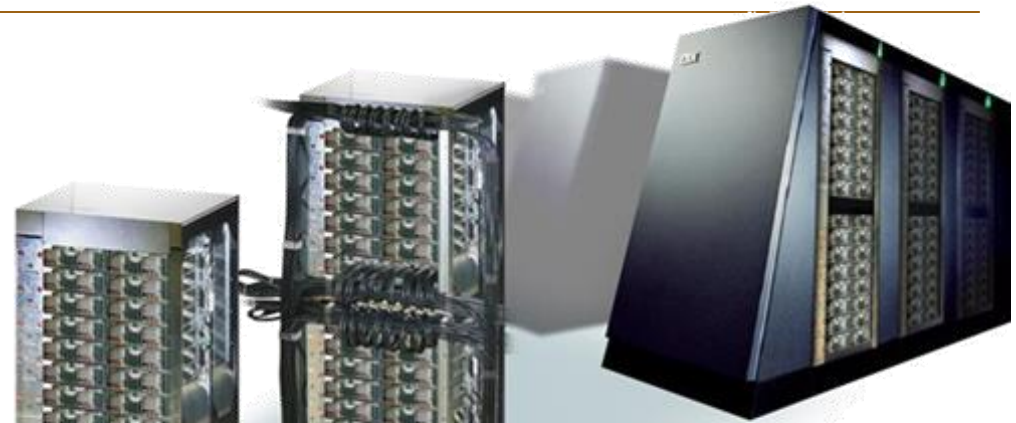
System 72 Racks, 72x32x32 1 PF/s, 144 TB
