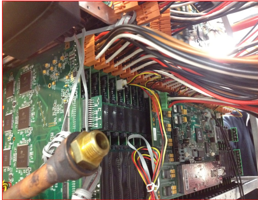
Figure 4.8 FECs fully connected with RCU and LV-power
