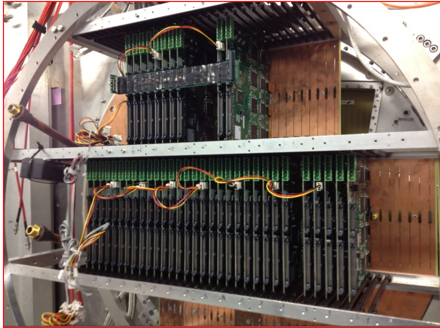
Figure 4.7 FECs connected to TPC
