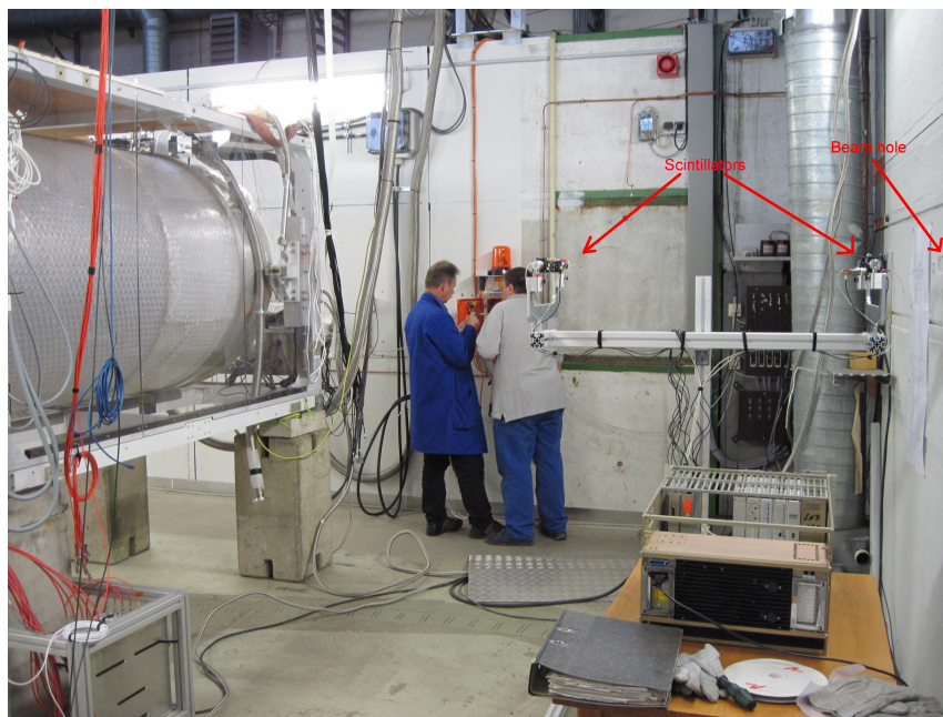
Figure 4.13: Four scintillators are used in coincidence to provide the trigger of an incoming electron. A measurement is started when all four scintillators fire simultaneously. The setup with four scintillators grouped two by two with a 100cm gap in between ensures that the a particle producing a trigger has to travel in the beam direction which minimizes the risk of an accidental triggering by e.g. a cosmic muon. By placing a delay between the two pairs it is also possible to get an estimation on the number of accidental coincidences.[38]
