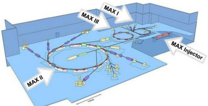
The accelerators at MAX-lab consist of three electron storage rings (MAX I, MAX II and MAX III) and one electron pre-accelerator (MAX injector). All three storage rings produce synchrotron light used for experiments and measurements in a wide range of disciplines and technologies. The MAX I ring is also used as an electrons source for experiments in nuclear physics.
