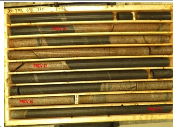
Granite drill cores around a candidate position
