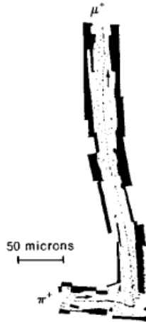
Figure 4.6: A photograph of a pion decay into a muon and a neutrino recorded in a nuclear photographic emulsion.
