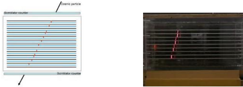
Figure 4.7: The general build up of a spark chamber (left) and a real track in a spark chamber (right).
