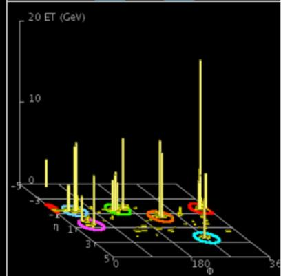
An event with 6 jets taken on April 4th, 2010. The jets have calibrated transverse momenta between 30 GeV and 70 GeV and are well separated in the detector.
