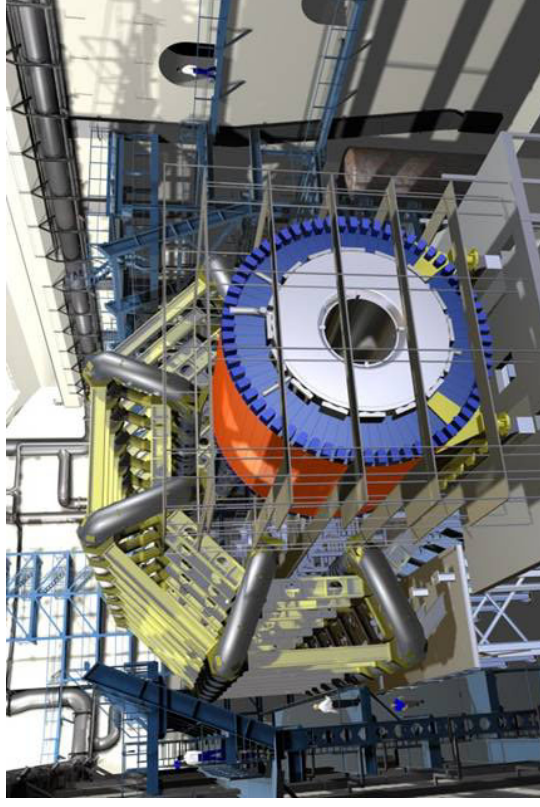
Engineering simulation: the Barrel Toroid and the Barrel Calorimeter installed in position (October 2004).
