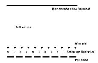
Electrons drifting along the electric field lines will be collected on the sense wires and produce a signal according to the same principle as for the MWPC. The charge cloud at the sense wire
