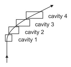
An alternative method is to keep the length of the cavities constant and change the RF-frequency of consecutive cavities.
