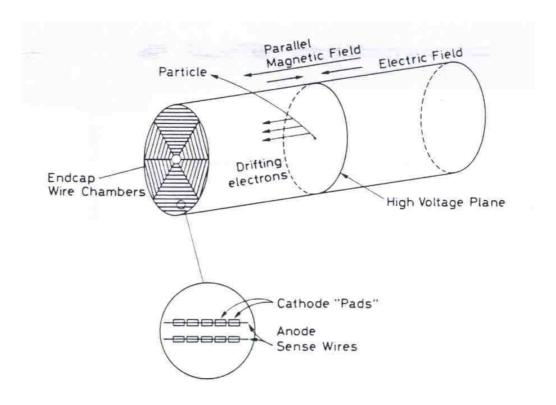
A closer look at the end plate (below) shows a *wire grid* plane followed by a plane of *sense*-and *field* wires and below these a *pad* plane.
