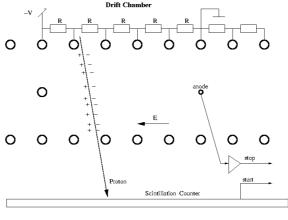
Drift Distance = Drift Velocity \* Time
