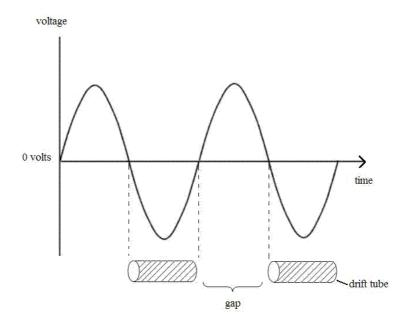
If the velocity of the particles is increased by every step of the acceleration, the particles will travel longer and longer distances during the acceleration time, which means that the lengths of the acceleration gaps and the drift tubes must be increased or alternatively that the frequency of the a.c. field is tuned to cavities of constant length.
