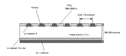
High resistivity n-type silicon is used as the starting material (wafer), i.e. the silicon has been doped with atoms containing an extra electron compared to the pure silicon and thus electrons are the majority charge carriers. Diod strips of p-type are implanted, where the doping atoms
