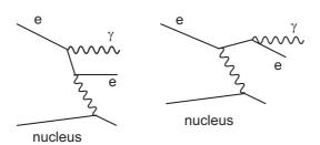
The photons will leave the accelerator, tangential to the beam orbit, through a thin window. The photons will not be monoenergetic but follow a specific momentum spectrum (bremsstrahlung spectrum).
