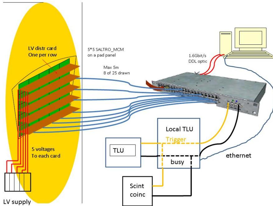
Figure 8: Schematic view of a serial readout system where an MCM-board communicates directly with the SRU via an interface card, which provides a transfer between the microHDMI and RJ45 cables.
