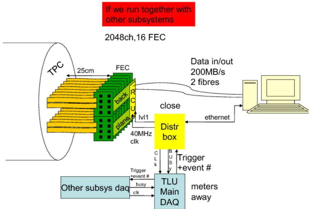
Figure 1: Schematic layout of the present readout system with the ALTRO electronics
