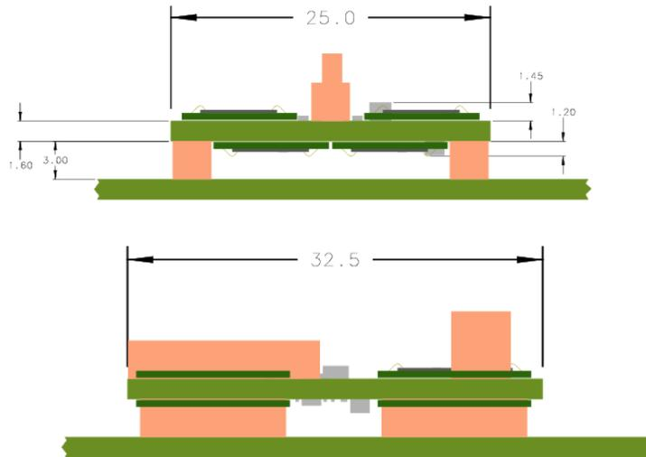
Figure 6: A schematic sideview of the board assembly.
