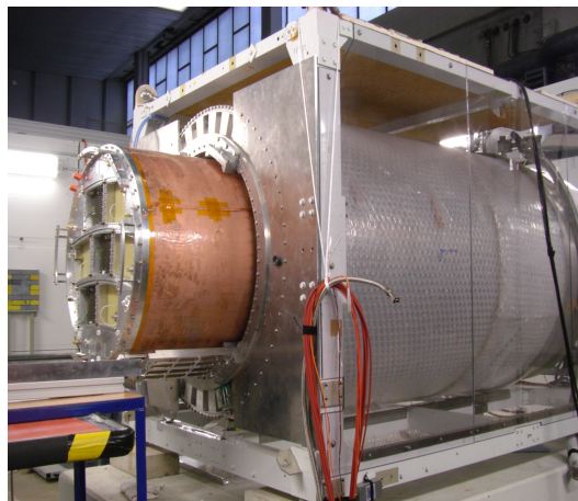
(b) The TPC field cage prototype at DESY half way into the magnet.
