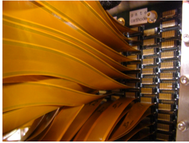
(a) Kapton cables connected to the pad connectors.
