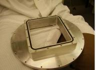
• Now the readout board is mounted. Four screws are left out where the longer screws, which hold the shield with the GEM stack, are inserted. At these positions the small spacer cylinders are placed.
