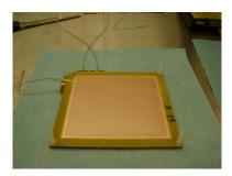
• Mount the last GEM with the copper coating and again arrange the connectors so they don't interfere with the other two GEMs. This time no spacer is needed.
