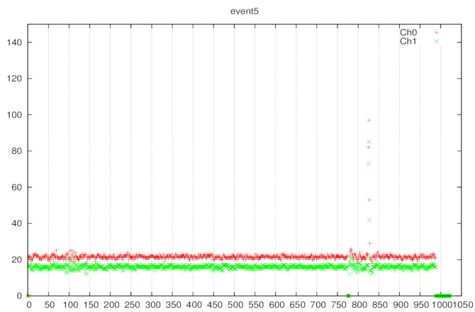
Figure 41: Readout of 2 channels with: a) 20MHz sampling clock b) 10 MHz sampling clock.
