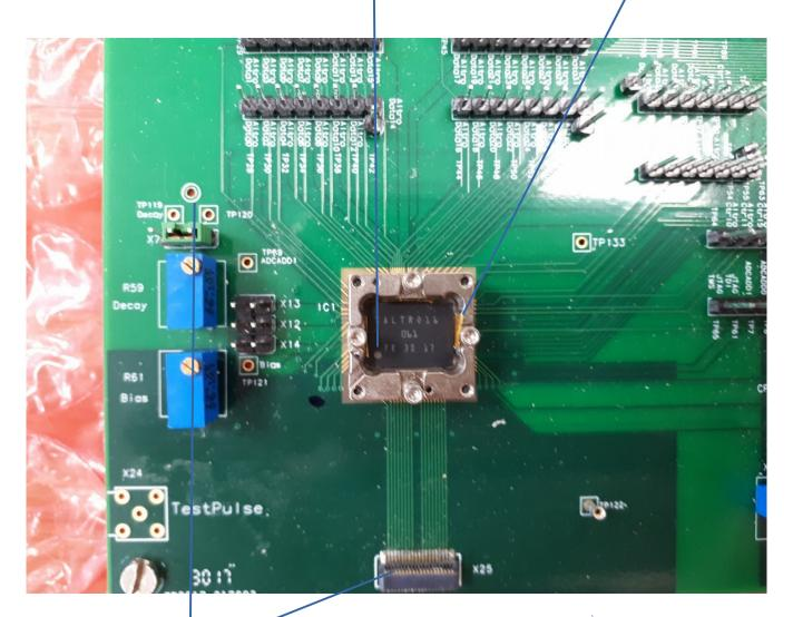
One can check that the re is connection by measuring the protection diode on the input to the preamplifier, connector X25. Use a multimeter with diodemeasure function, with common ('-') to the input and V ('+') to ground. This should give a value of 0.8.
