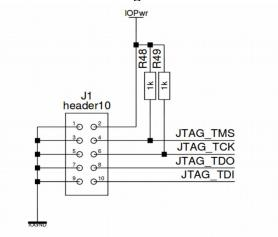
To the card do we have a connector onto which the individual signals are connected for the ease of insterting/removing the the individual cables: (each individual cable is labled).
