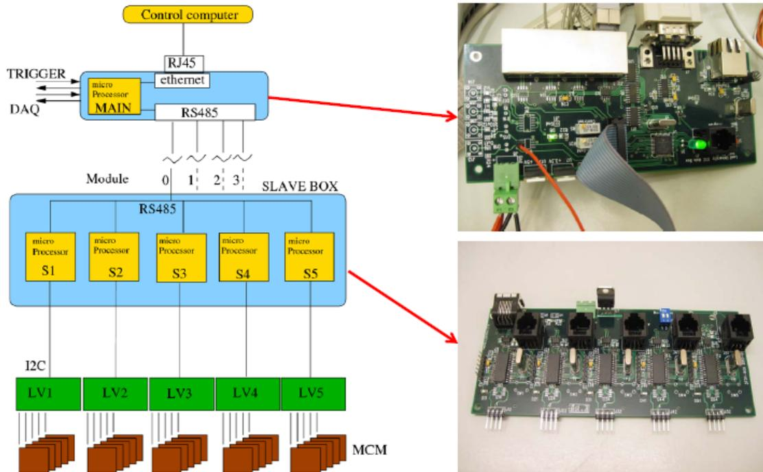
Figure 9: A schematic view of the Detector Control System (left) and the corresponding boards (right).
