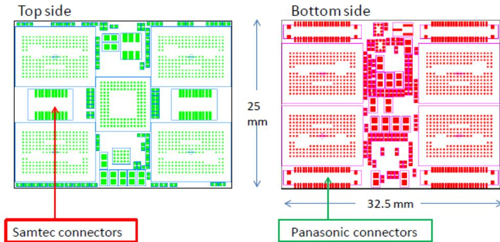
Figure 4: *The MCM-board top surface (left, green) and bottom surface (right, red)*
