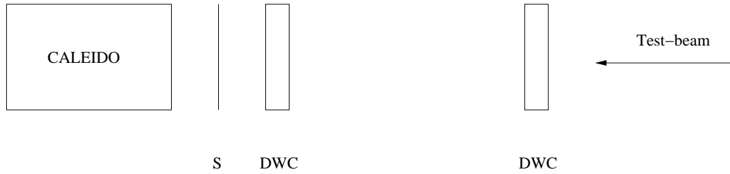
Figure 4.5: The test-beam setup at the CALIEDO test run.
