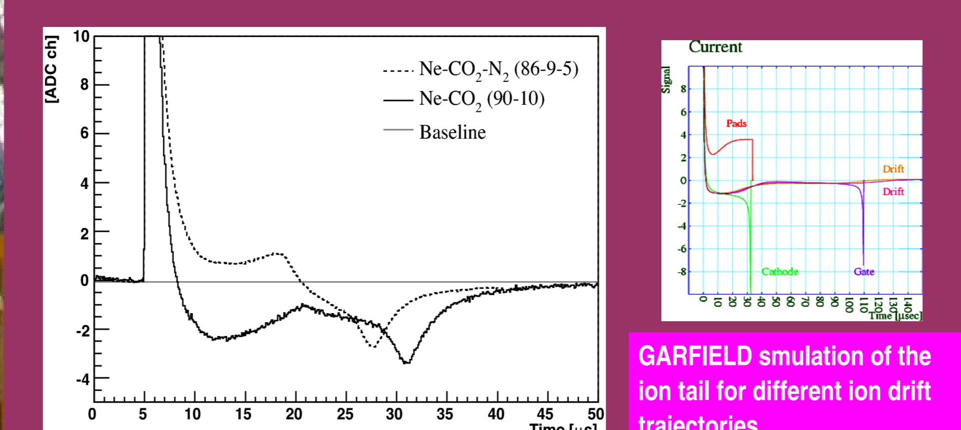
The ion tail was measured for clusters with large signals. It was slightly different for the two gas mixtures:
