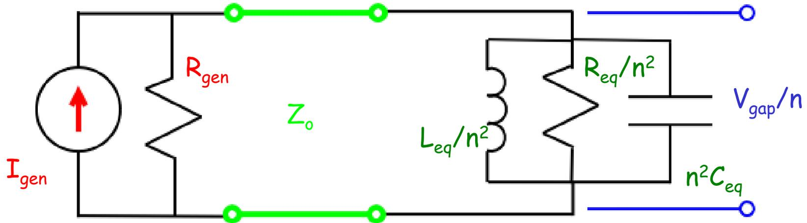
Assume that the power amplifier is matched ( $R_{gen} = Z_o$ ) and define a coupling parameter as the ratio of the real part of the cavity impedance as seen by the power amplifier to the characteristic impedance.
