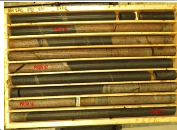
Granite drill cores around a candidate position
