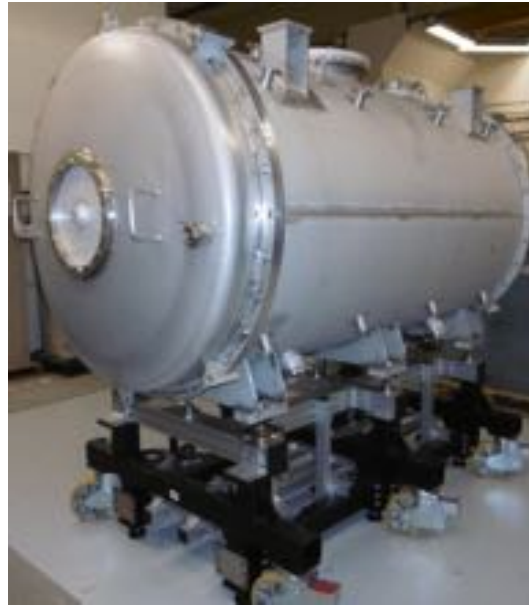
Vacuum vessel & Mechanical support
