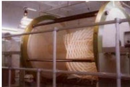
If the drift chamber is placed in a homogenous magnetic field the momentum,  $p$ , of the particle can be determined from the measured curvature of the trajectory according to the relation:
